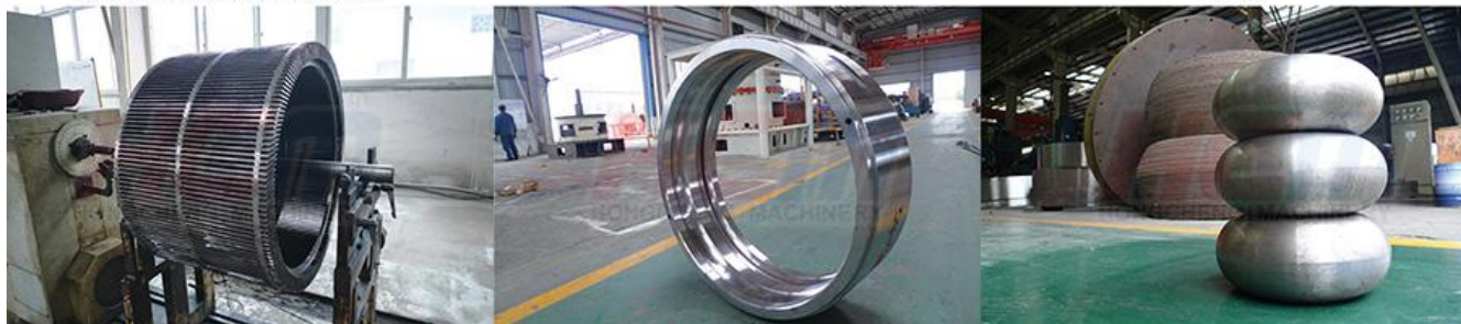
Dynamic balance test is carrying out to the rotor of the Classifier
